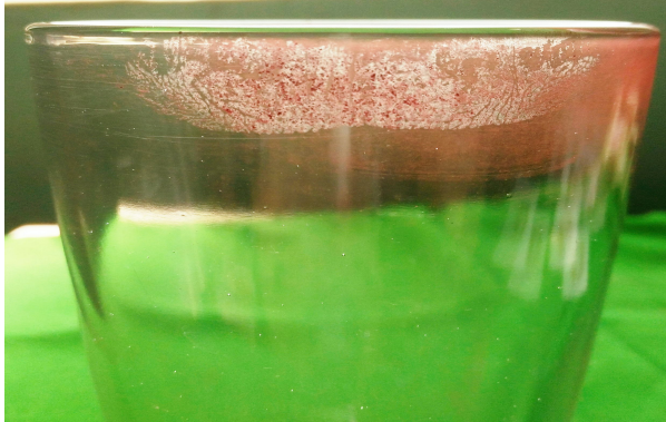
Fig. 10: Latent lip print developed by Sudan III on glass tumbler
