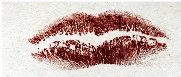
Fig. 2: Latent lip print developed by Sudan III on bond paper
