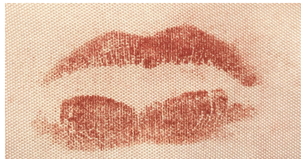
Fig. 6: Latent lip print developed by Sudan III on satin fabric
